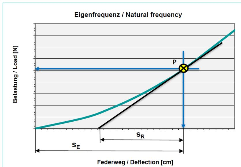
$$\text{Natural frequency [Hz]} \quad fe = \frac{5}{\sqrt{sR}}$$
