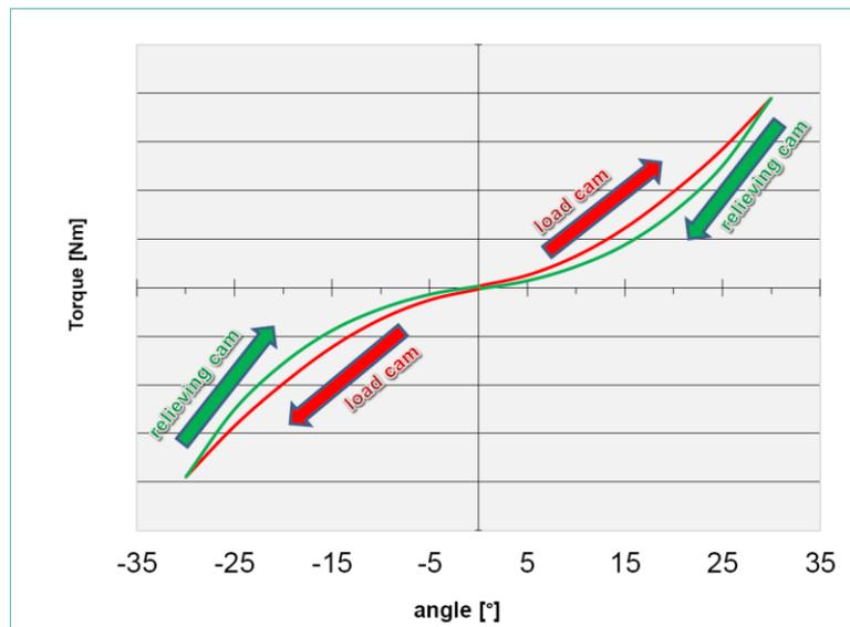
All elastic materials have a measurable settling and a compression set (DVR). This means that rubber give way in the load direction depending on the time, the load, the load change, the excitation frequency and the temperature after discharge not goes more fully back to the initial position.
