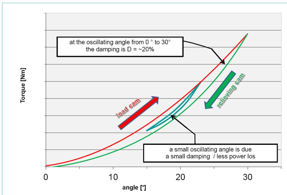
The result is a larger damping at a large torsion angle with less excitation frequency. Adverse shocks and vibrations are reduced in a few deflections.
