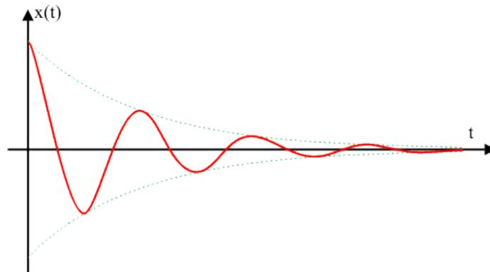
It results a small damping at a small oscillating angle with high excitation frequency. In operation with harmony-excited oscillations, only a small proportion is converted to heat. As soon as the amplitude peak to peak increases up in case of the resonance passage to the maximum of 2.3 times higher, the oscillating is reduced in a few deflections by increasing damping.
